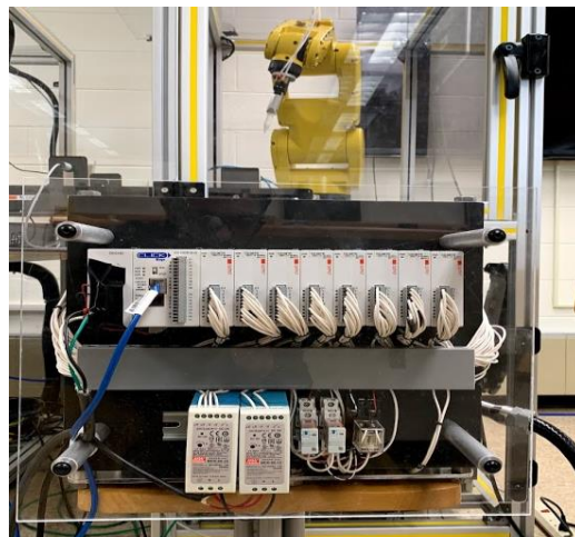
Figure 2: The final setup of remote robot system with FANUC LR-Mate 200iC robot and CLICK PLC
