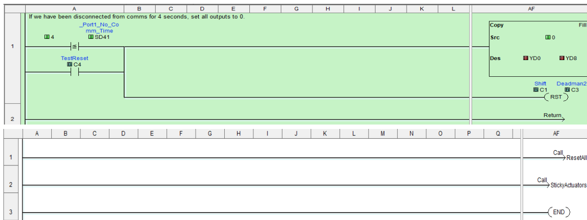
Figure 8: Security of SHIFT and Deadman Switch by using Reset All block for resetting the system if servers are disconnected for 4 seconds.
