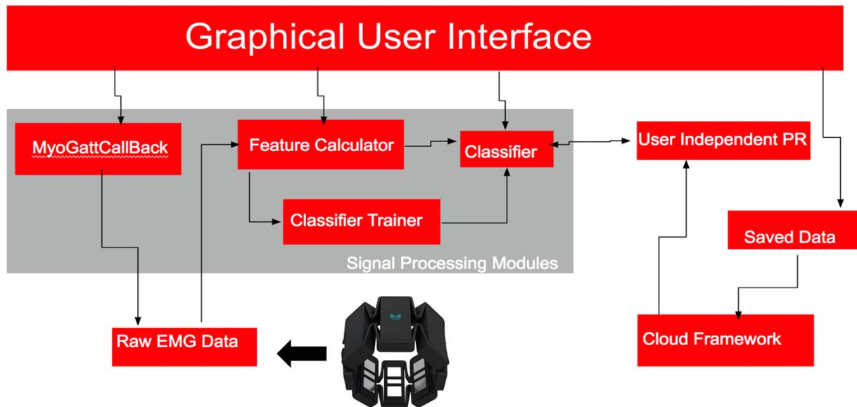
Figure 1. Overall structure of the Android application
