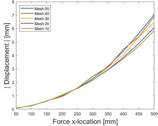
Figure 5. 2D plot on beam deflection under point loads with different mesh sizes
