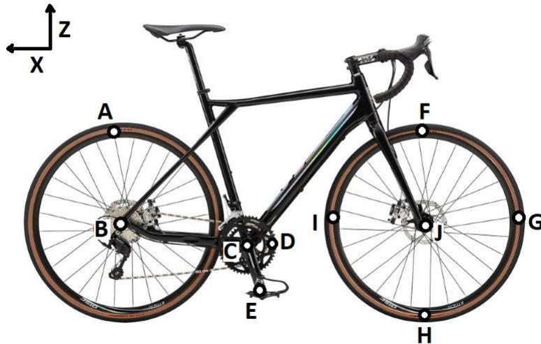
You will be analyzing the motion of various components on a typical bicycle. Using the HMB Lab, we will give you the x-y positions (in mm) of different markers shown in the image above as a function of time. Markers A-B define the rear wheel, markers C-D-E define the bicycle crank, and markers F-G-H-I define the front wheel.
